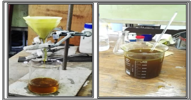
Fig. 4 The prepared ferric chloride solution ( \text{FeCl}_3 \cdot 6\text{H}_2\text{O} ) during filtering
