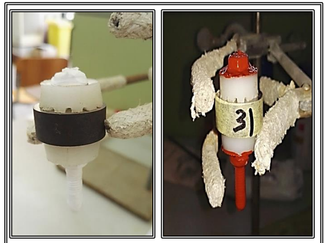
Fig. 5 Protecting operations of bolt, nuts and flat washers against corrosion
