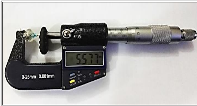
Fig.6 Crevice depth evaluation process
