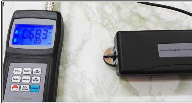
Fig. 2 The surface roughness measurement device
